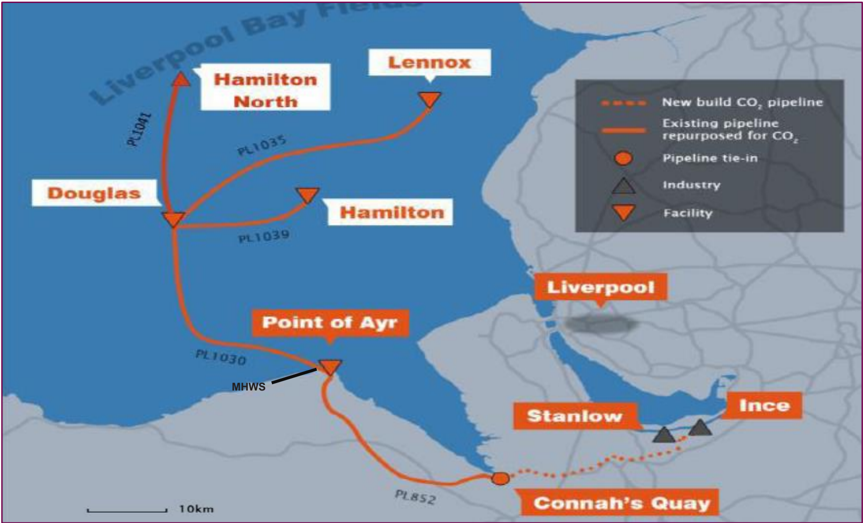
Figure 1.2: Illustrates The Concept Of The Proposed Development (Infrastructure Seawards MHWS)
