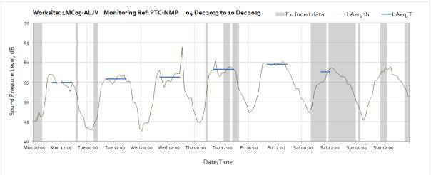
Note: Missing data on 4<sup>th</sup> of December at 11:00 was due to monitor field calibration.
