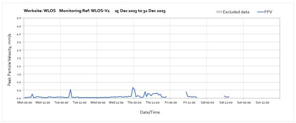
Note: Intermittent missing data throughout the week until the end of the month was due to poor weather conditions and vegetation growth effecting the solar power source to the monitoring station.
