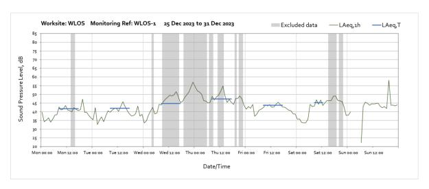
Note: Missing data between 02:00 and 06:00 on Sunday 31<sup>st</sup> December was due to poor weather conditions and vegetation growth effecting the solar power source to the monitoring station.
