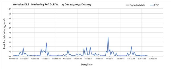
Note: Missing data from 07:00 on Sunday 31<sup>st</sup> December until the end of the month was due to poor weather conditions effecting the solar power source to the monitoring station.
