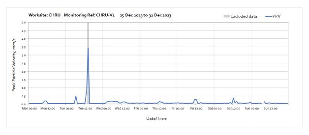
Note: Missing data between 07:00 and 08:00 on Sunday 31st January was due to poor weather conditions and vegetation growth effecting the solar power source to the monitoring station.
