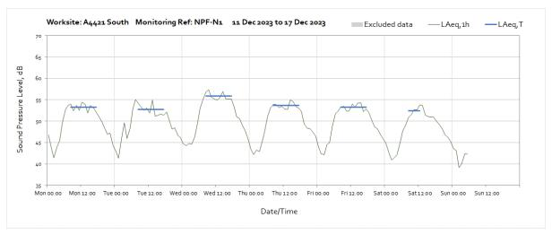
Note: Missing data between 06:00 on Sunday 17<sup>th</sup> December until 12:00 on Monday 18<sup>th</sup> December was due to insufficient power provide by solar panel supply following a period of sustained poor weather.
