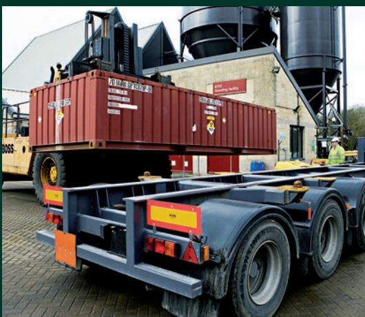
TC01 at the Repository site grouting facility, each container is filled with grout to create a solid structure, suitable for disposal in our vaults
