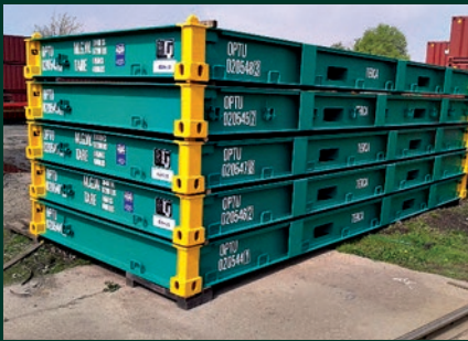
Collapsible flat racks (ISO platform container) shown stacked five high for transport
