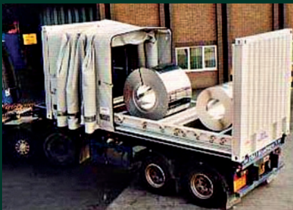
ISO platform container fitted with sliding cover for weatherproof transport
