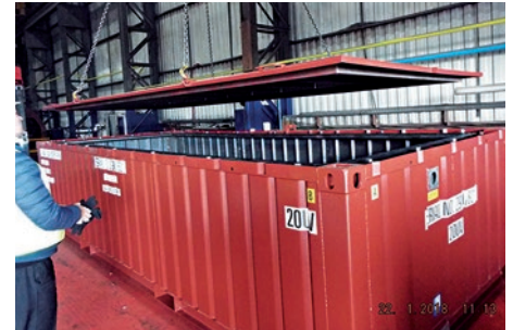
TC01R lid being lifted off using an overhead crane and four-chain sling
