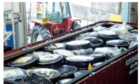
Drums after supercompaction at treatment facility loaded in a half height ISO container
