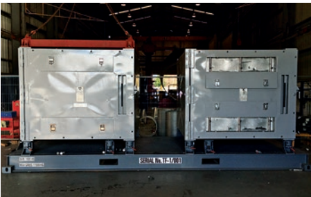
2x Novapaks restrained onto the dedicated Novapak Transport Frames
