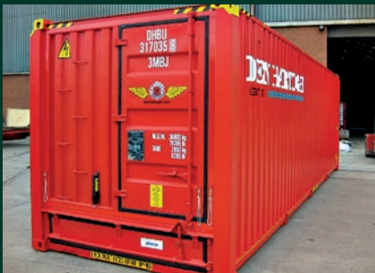
Modified full height ISO container with end wall access on one side only
