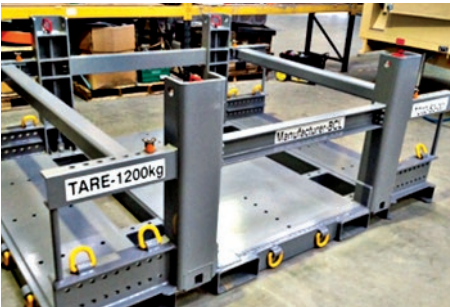
S3 half size stillage fitted with restraint bars for transportation of drums
