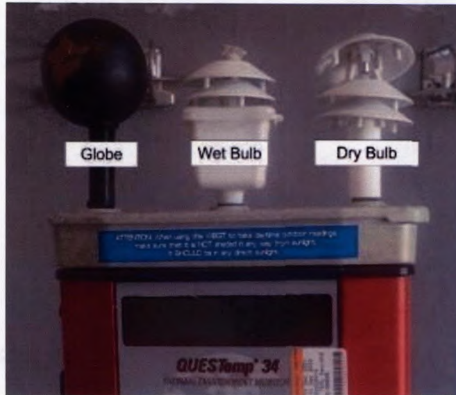
Figure 1.4.2 - Damaged QT34 instrument
