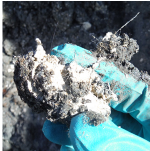
Degraded asbestos debris in soil | AECOM
