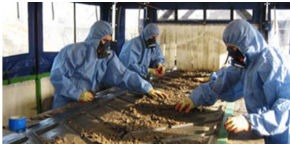
Hand picking of asbestos fragments on a belt | McAuliffe
