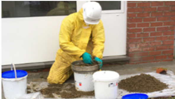
Asbestos sampling activities in Belgium | AECOM
