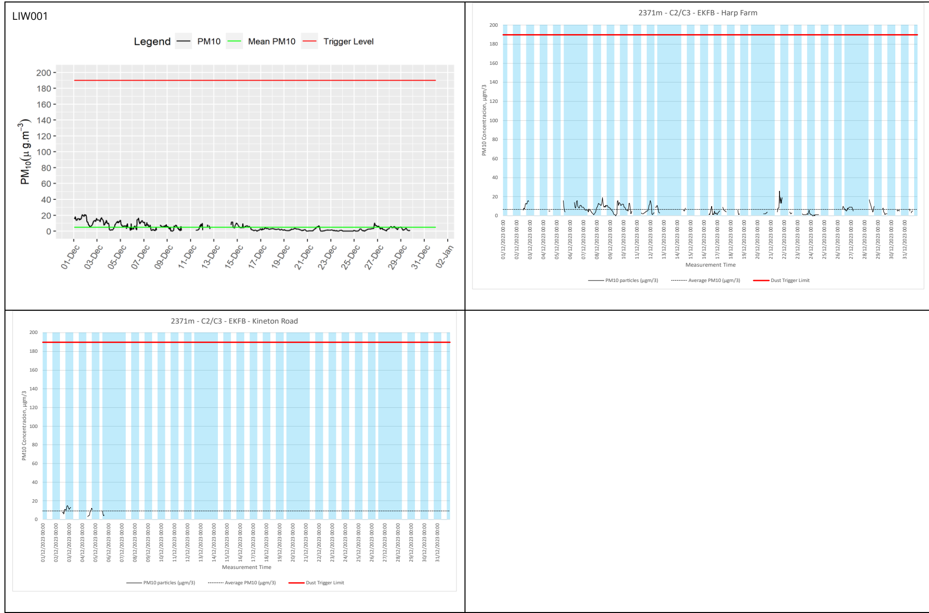
Figure 2: Construction dust 1-hour mean indicative PM 10 concentration for all dust monitors
