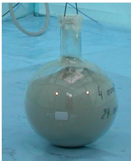
Figure 2: Experiments comparing RF for different drop heights from glass container containing PFA powder (from Fig 3.1 of [9]; results plot from Fig 4.3 of [9] – note the break in the ordinate (Y-axis), where the scale at the top and bottom of the plot are different)
