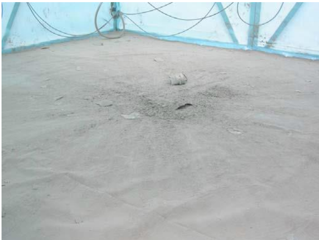
Figure 4: Experimental result for glass container containing 10 kg of PFA powder dropped from 9 m (from Section 10.2.1.1 of [11])
