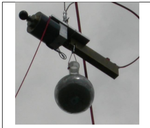
Figure 4: Lifting and glass specimen release mechanism [8]
