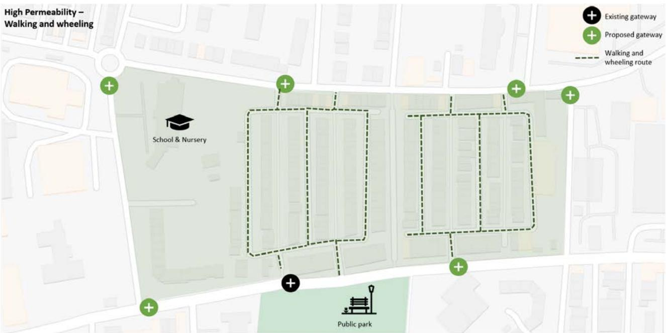
**Figure 12 – Example of high walking and wheeling permeability – Multiple routes with all of the features from the list**
