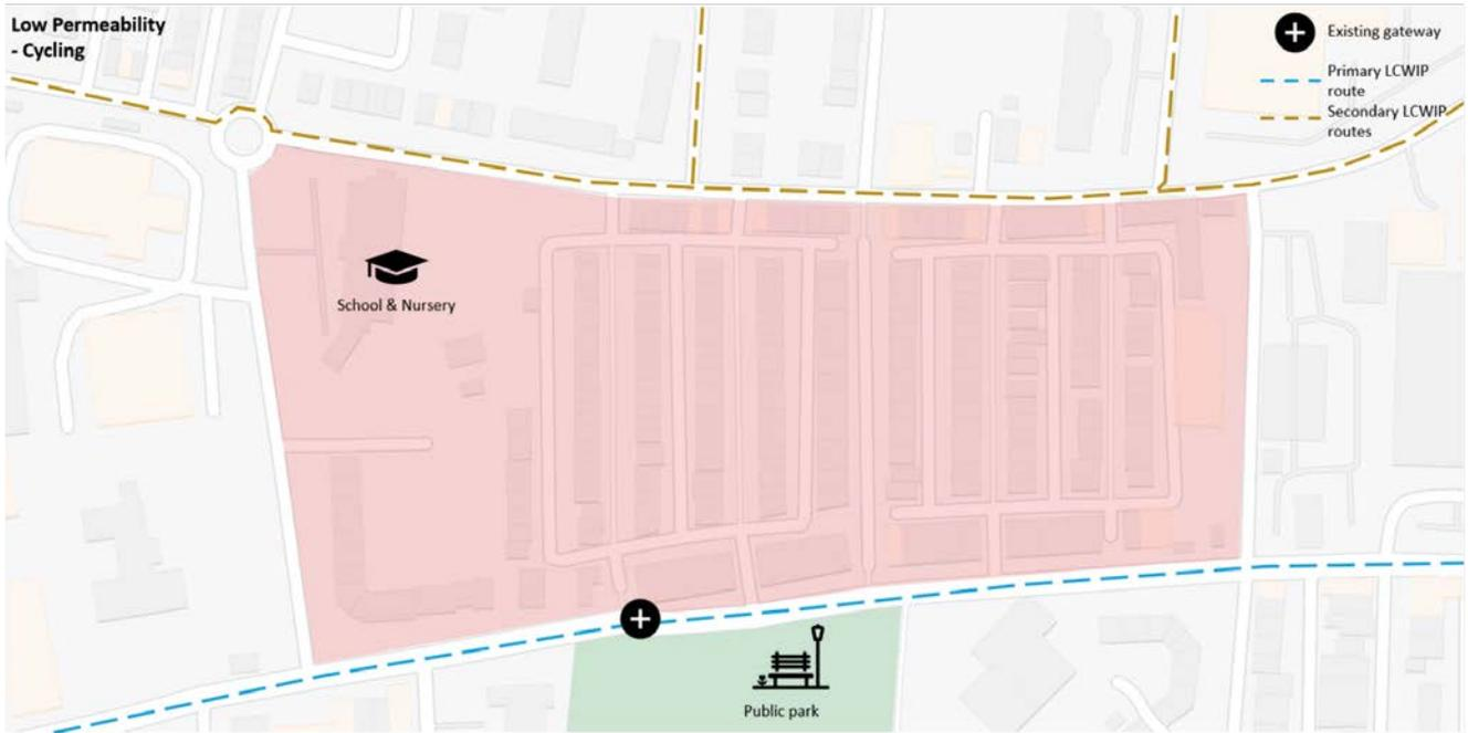
**Figure 13 – Example of low cycling permeability – No routes through the area**
