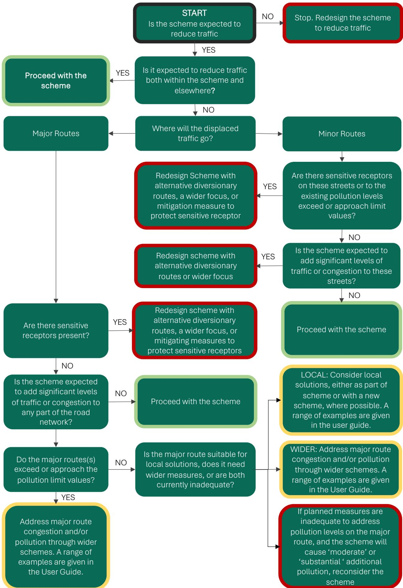
Figure 8 – Flowchart illustrating the logic of the Traffic Mitigation Check
