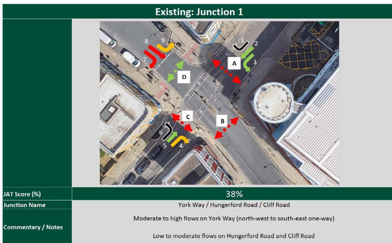
**Figure 14 – A completed JAT Diagram for the existing situation at a junction, using satellite imagery from Google Maps**
