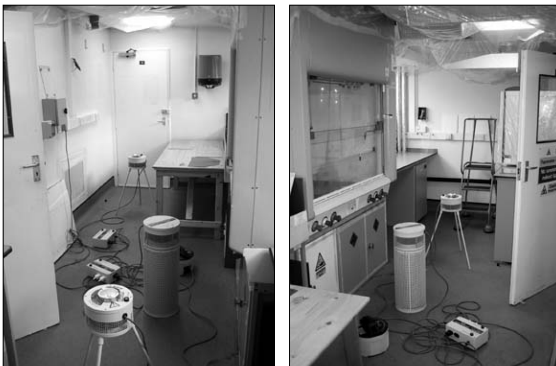
Figure 5: 40m 3 room used for the trial. The SUPERfume equipment is shown set-up prior to the experiment
