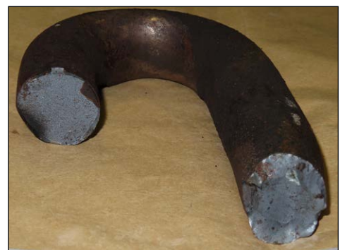
Figure 2: Failed chain link on Honeybourne III
