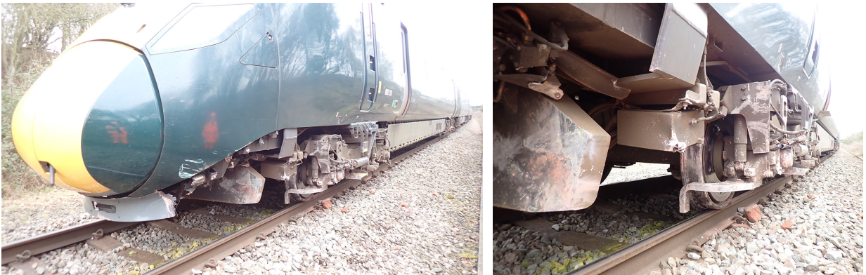
Figures 9a and 9b showing damage to the front of the train.
