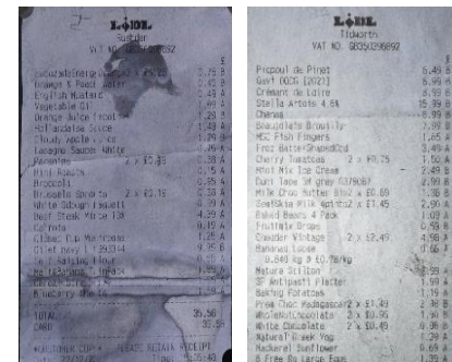
Figure 6. Example of Lidl receipts processed with acetone wash and Indandione (left) and Indandione only (right). Both receipts were left to develop in the dark (no FDO).
