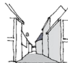
(Top)- Width of space equal to or less than height of enclosing planes. (Bottom) Drop in height at (a) compensated by rise in height on opposite side
