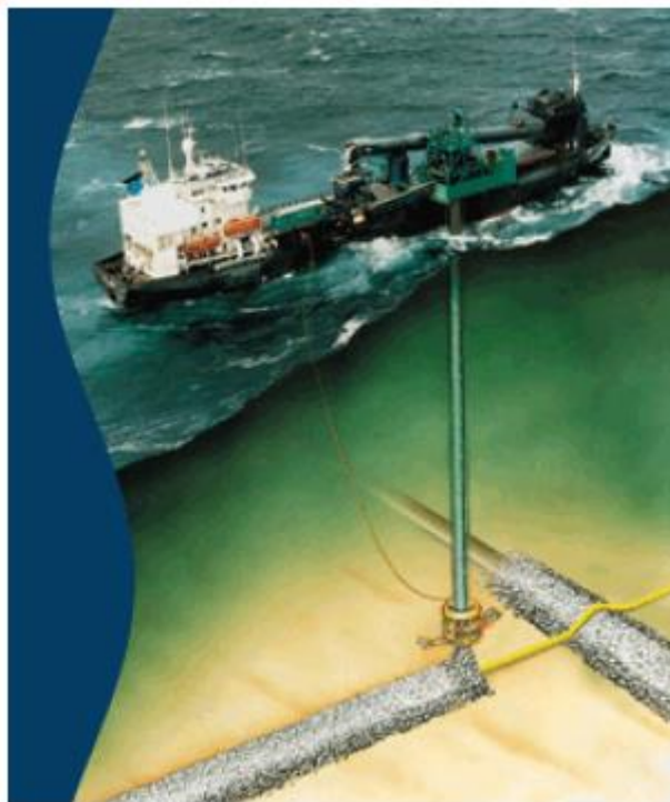
Figure 4-3 – Remedial Rock Cover Installation Illustration
