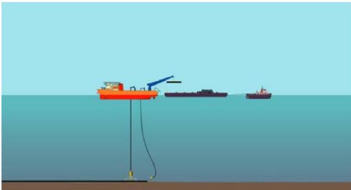
Figure 4-1 – Cut and Lift Pipeline Removal Illustration
