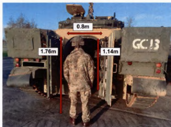
Figure 1.4.22 – FV511 rear door opening dimensions
