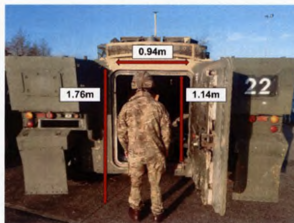
Figure 1.4.23 – FV510 rear door opening dimensions
