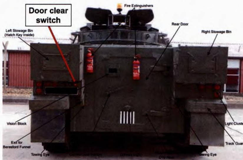
Figure 1.4.17 – FV510 'door clear' switch
