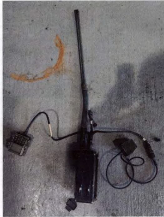
Figure 1.4.41 – PRC 354 radio and folded 1.5m whip antenna
