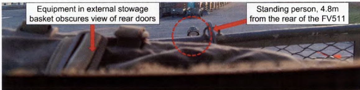
Figure 1.4.47 – An FV511 commander's view through a rear periscope with rear doors open (turret facing forward and equipment in external stowage baskets)
