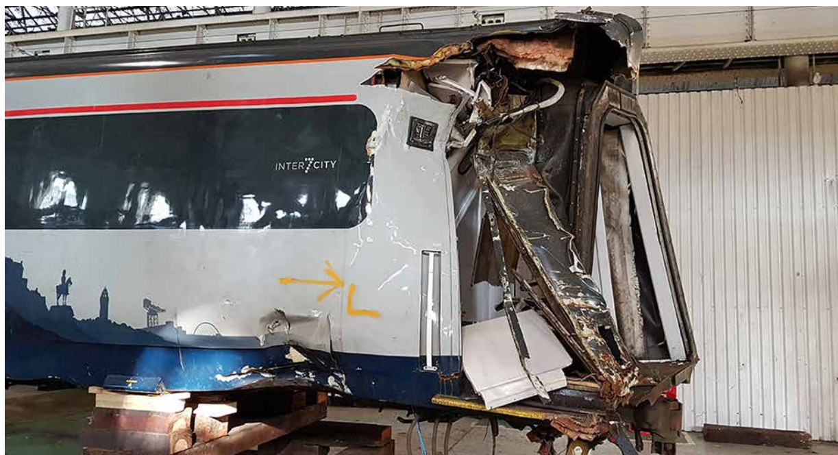
Figure 79: Damage to leading end of coach A
