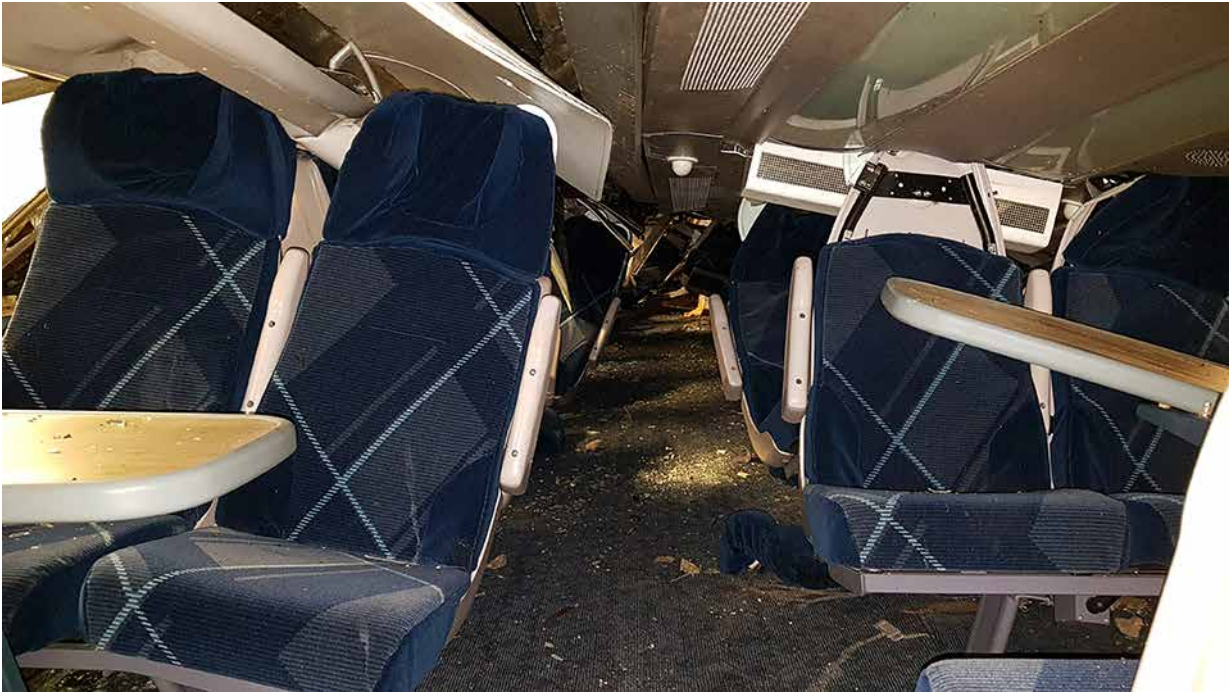
Figure 75: Interior damage at leading end of coach D
