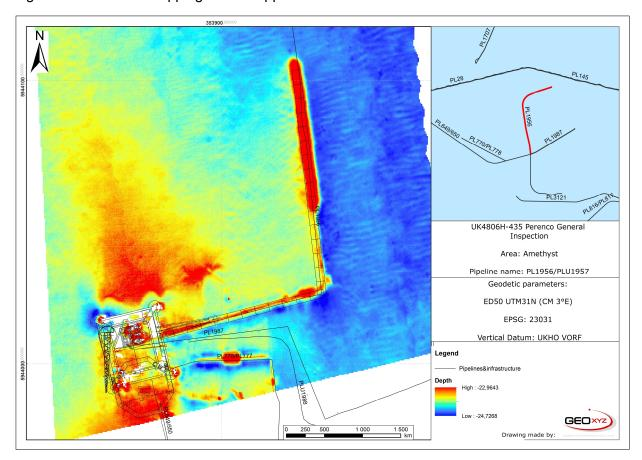
Fig A.7 2022 MBES mapping of A2D approaches
