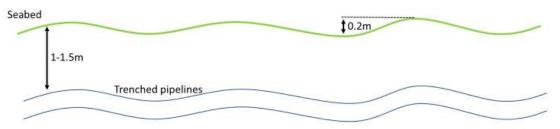
Trenched pipeline profile tends to match seabed profile above it.
