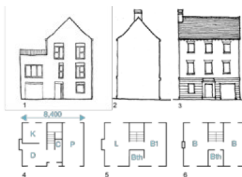
1. Front elevation 2½ storey 2. Side elevation 3 storey 3. Front elevation 3 storey 4. Ground-floor 5. First-floor 6. Second-floor
