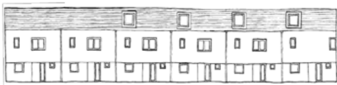
Front elevation with larger openings and facade subdivided to emphasise individual houses
