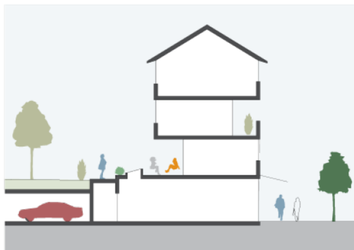
Single-aspect ground-floor uses with rear under-deck access
