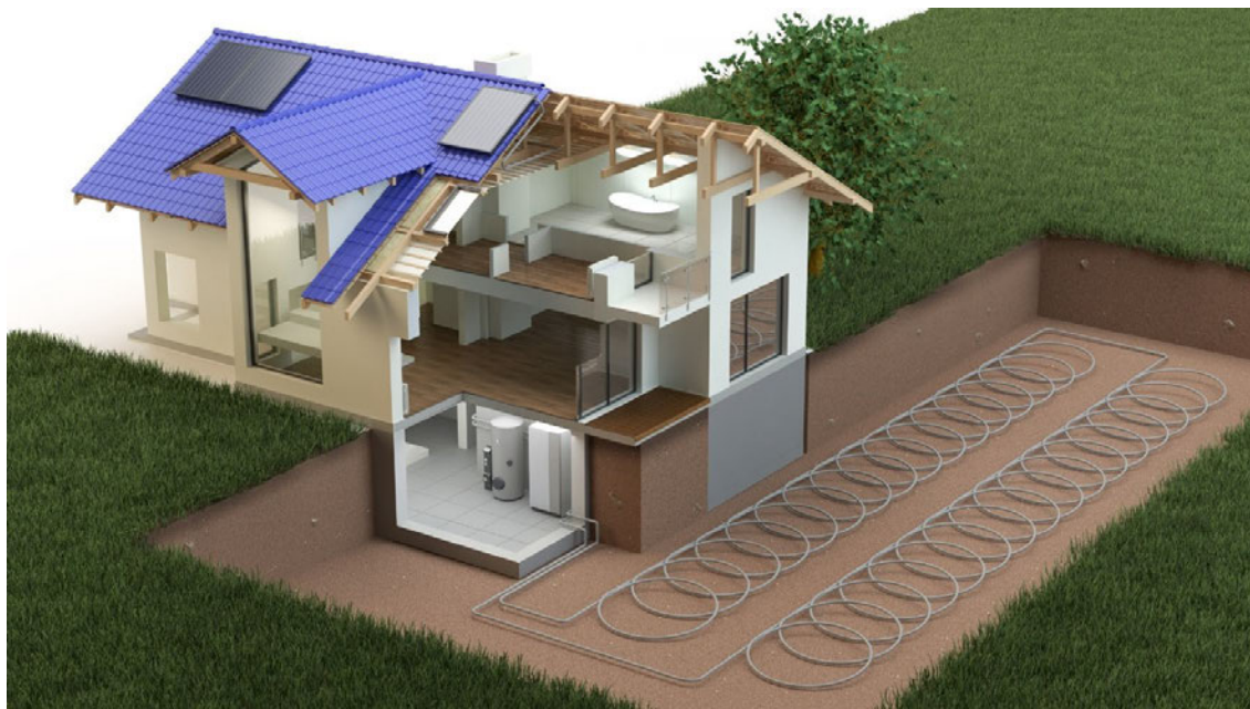
Horizontally sunk ground source heat pump
