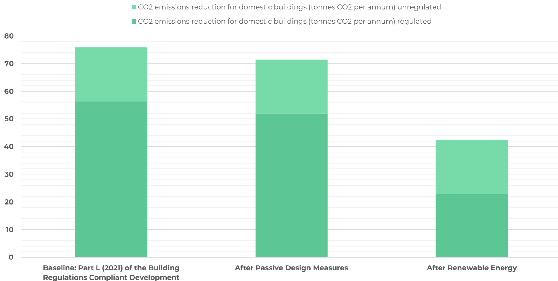
Figure 5: Total site-wide savings at each stage of the energy hierarchy
