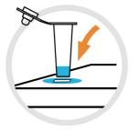
6 Place the extraction tube containing the buffer in the extraction tube holder hole in the box.
