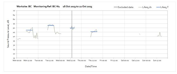
Note: Missing data throughout the week was due to vegetation obscuring solar panels leading to a loss of monitor power.
