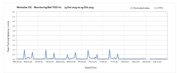
Note: Missing data between 00:00 and 01:00 on Sunday 29th October was due to a monitor time adjustment at the end of British Summertime. In the period 02:00 to 04:00 following the time adjustment much data was missing and this is attributed to clock synchronisation problems.
