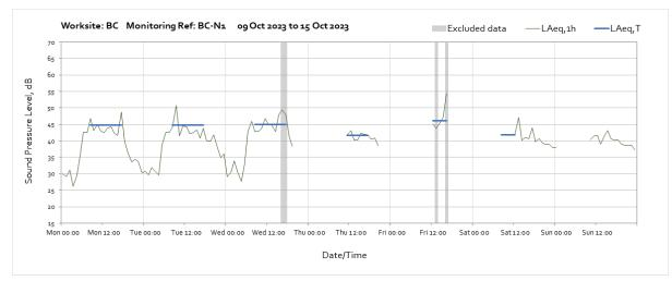
Note: Note: Missing data throughout the week was due to vegetation obscuring solar panels leading to a loss of monitor power.
