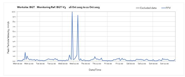
Note: The high vibration levels on Wednesday 18<sup>th</sup> October are due to concrete pouring and utility diversion works.
