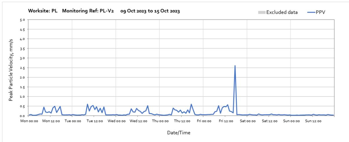
Note: High vibration level between 17:00 and 18:00 on Friday 13<sup>th</sup> of October was due to stockpiling of material and plant movements.
