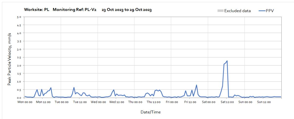
Note: High vibration levels between 10:00 and 13:00 on Saturday 28<sup>th</sup> of October was due to stockpiling of material and plant movements.
