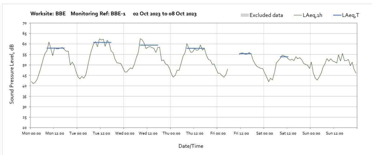
Note: Missing data between 06:00 and 11:00 on Friday 6<sup>th</sup> of October was due to over grown vegetation blocking the solar panels for battery power to the monitoring station.
