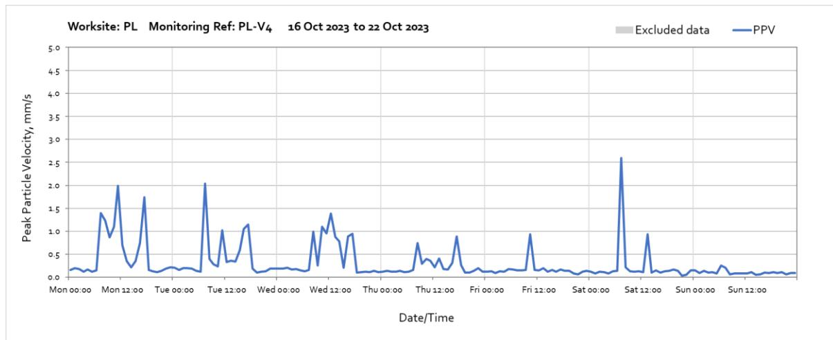
Note: High vibration levels between throughout the month were due to piling works.
