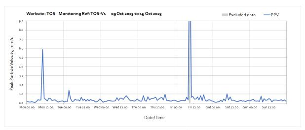
Note: High vibration levels between 09:00 and 10:00 on Monday  $9^{th}$  of October were due to sewage treatment plant works within 53m of the monitor.
