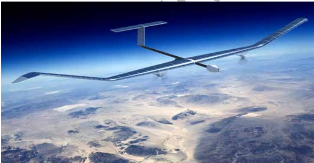
Persistent high altitude pseudo-satellites – the solar powered Zephyr remotely piloted air system flying in the stratosphere
