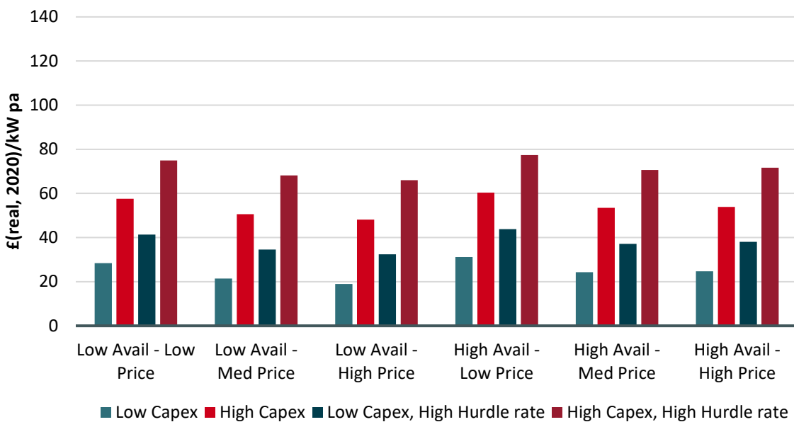
Figure 47: CM support required for new build CCHT commissioning in 2026 assuming hydrogen blend
