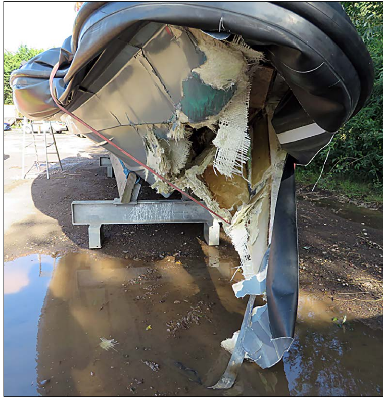
Figure 15: Damage to the bow of Seadogz
