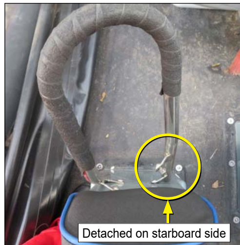
Figure 17: Jockey seat J1 handhold detachment
