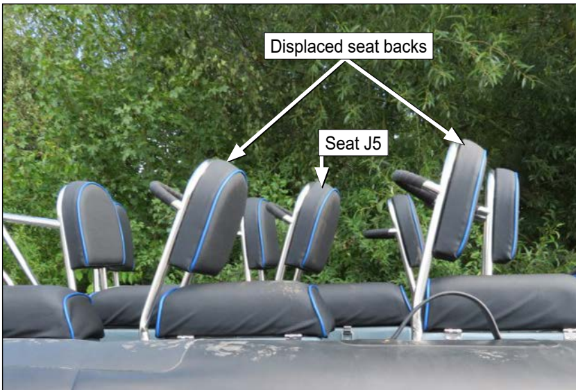
Figure 16: Damage to the backs of the jockey seats on board Seadogz following the accident
