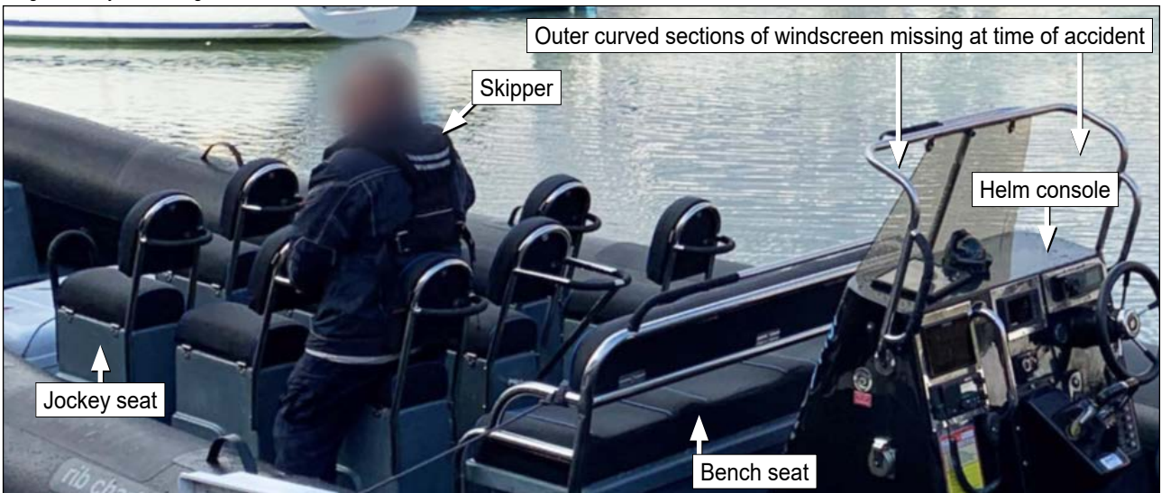
Figure 2b: The cushioned seats on Seadogz and the skipper demonstrating how to sit on a jockey seat
