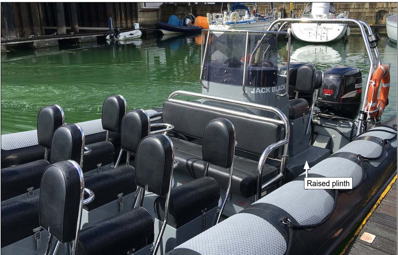
Figure 29: Example of raised plinth helm station as found on Jack Black
