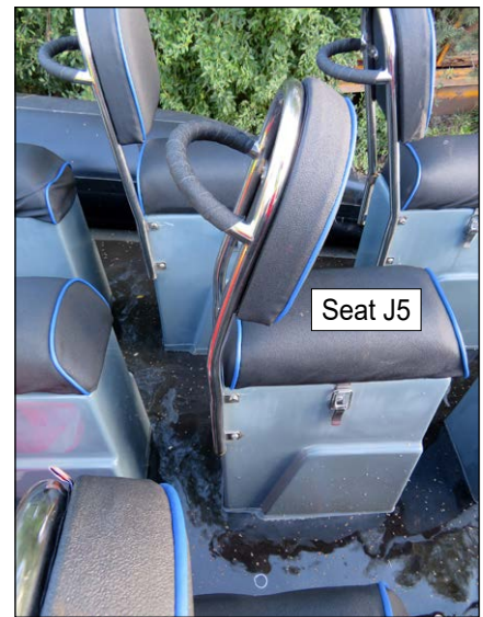
Figure 16: Damage to the backs of the jockey seats on board Seadogz following the accident
