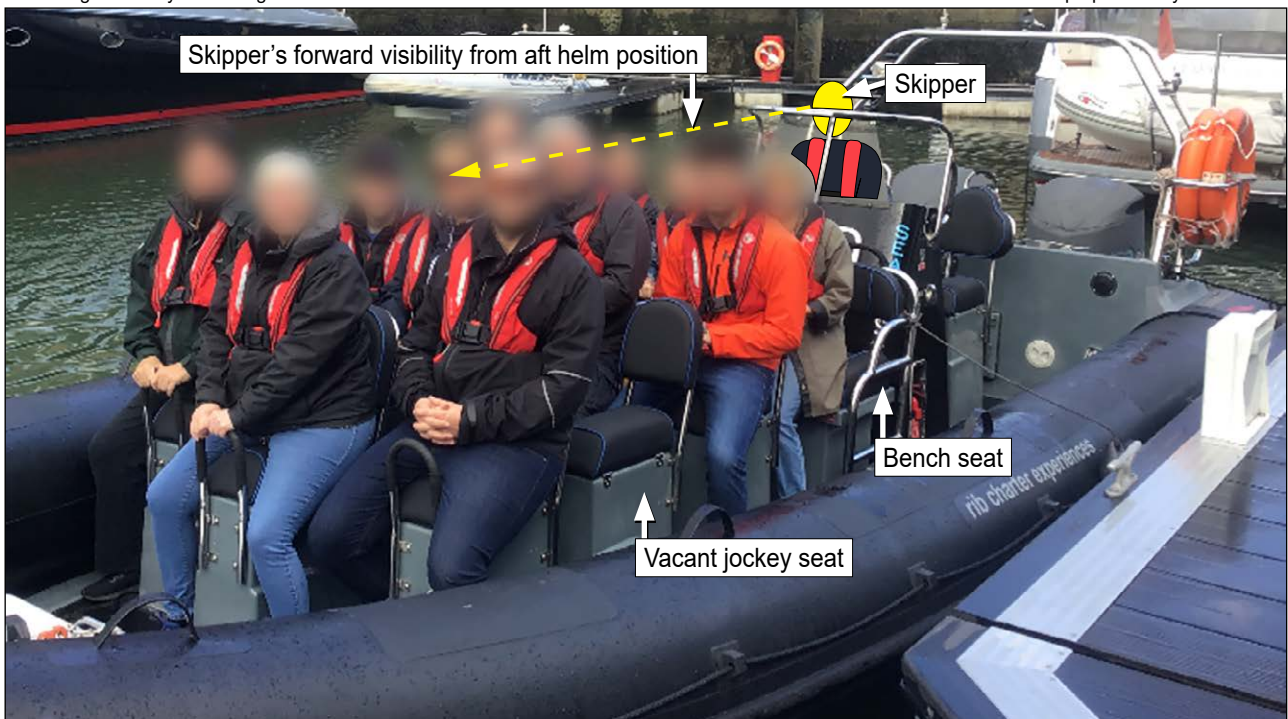
Figure 21: Representation of skipper's forward view being obscured by the seated passengers
