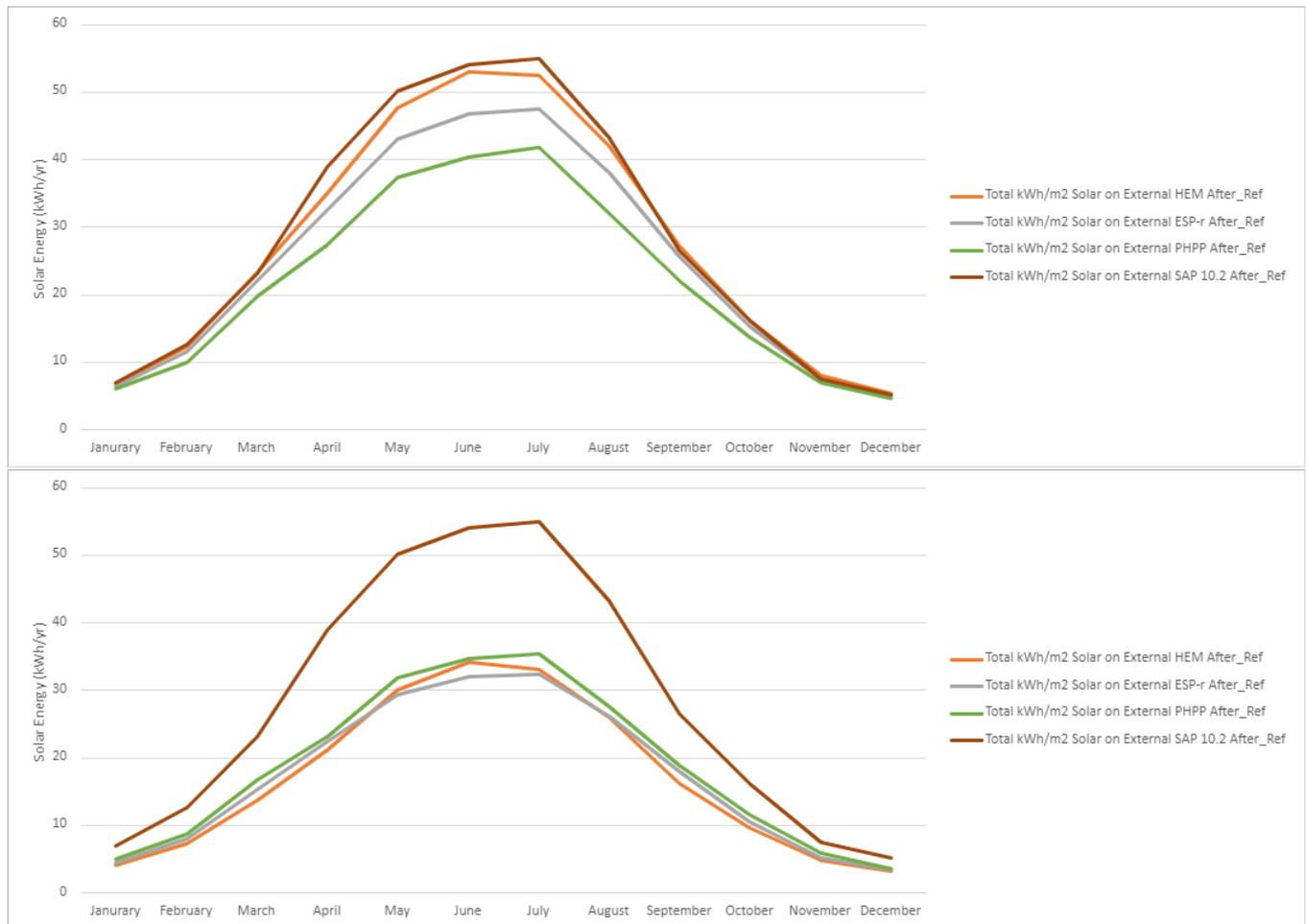
**Figure SB2 – Shoebox comparison of total monthly shortwave solar radiation entering through North facing transparent element (Above – no near shading; Below – with near shading)**
