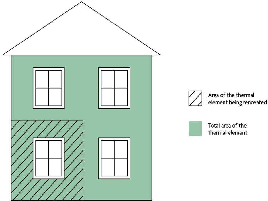
Diagram 12.1 Renovation of a thermal element from the outside
