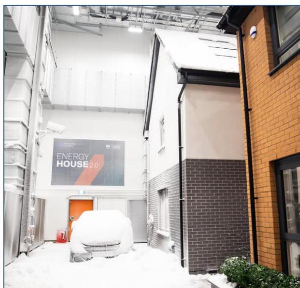
Energy House 2.0 is a world leading energy performance test facility at the University of Salford. It contains two environmental chambers each able to accommodate two detached houses and under controlled conditions, recreate a wide variety of weather conditions with temperatures ranging between -20 °C to +40 °C and simulated wind, rain, snow and solar radiation.
