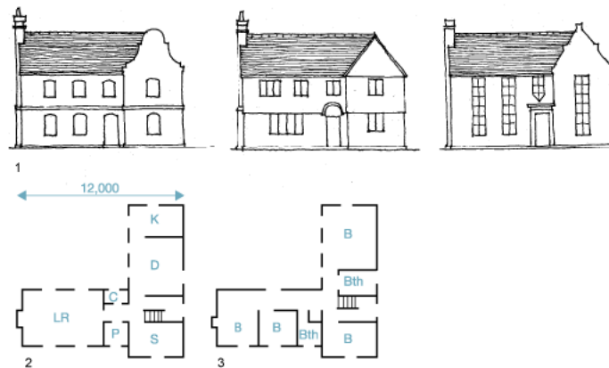
1. Front elevations 2. Ground-floor 3. First-floor
