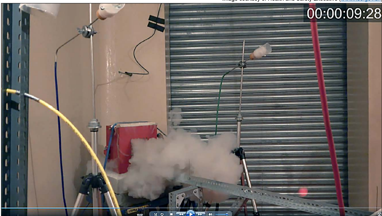
Figure 20: Set up of HSE condensed aerosol generator test
