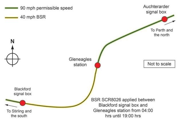
Simplified diagram showing location of the blanket speed restriction. Not to scale and not all features shown.
