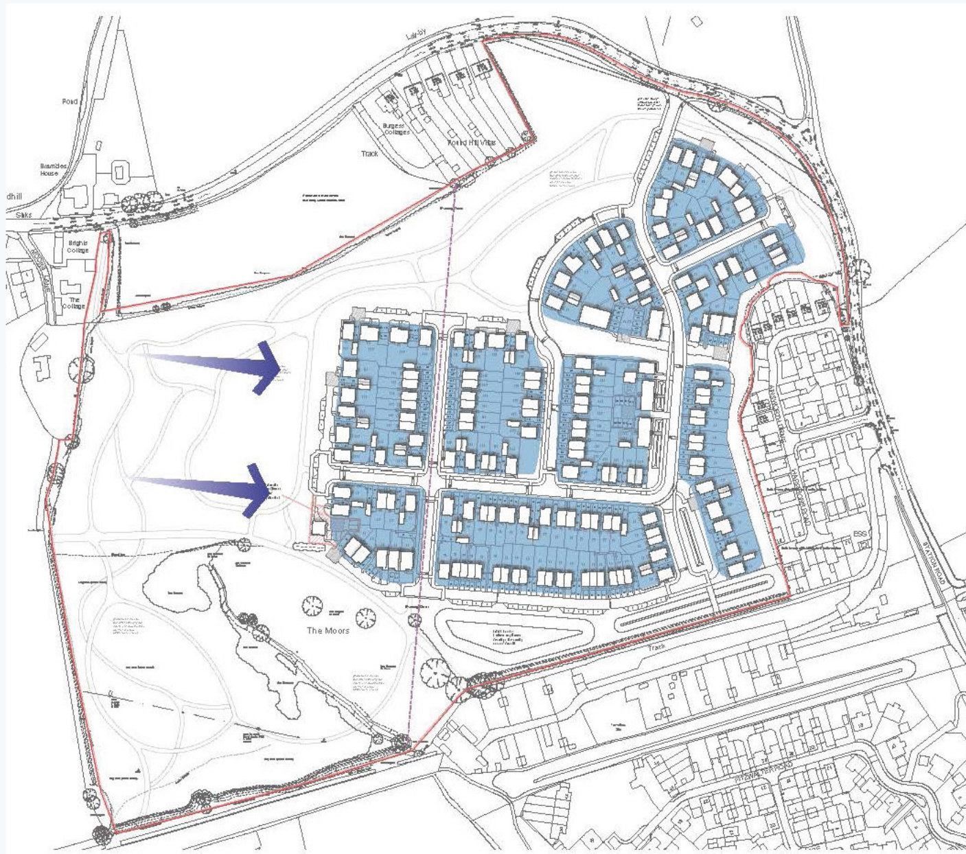
LAND PARCELS SET BACK FROM WESTERN BOUNDARY TO REDUCE NEGATIVE HARM TO HERITAGE ASSETS
