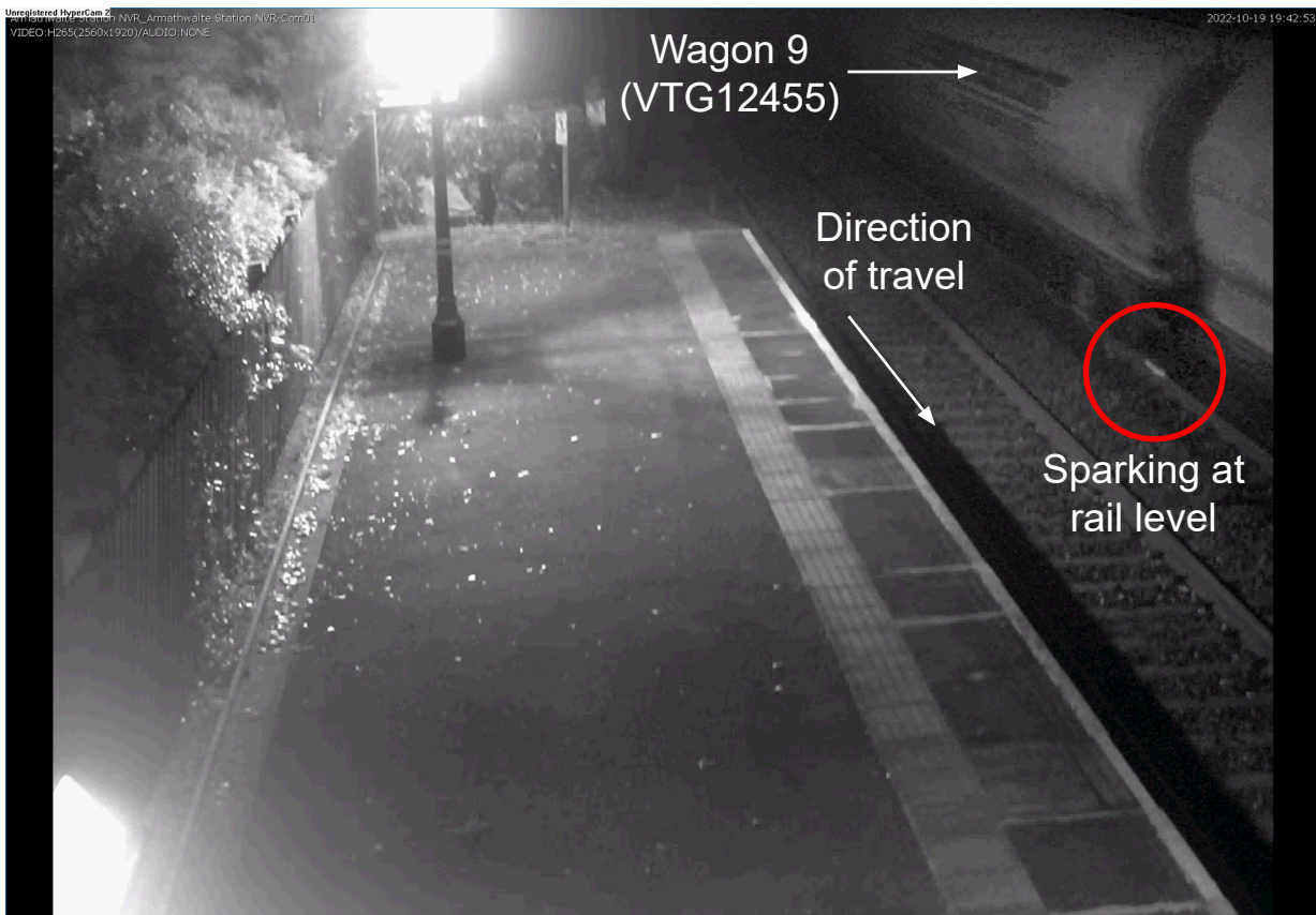
Figure 19: Sparking from the ninth wagon in train 6C00 at Armathwaite station (courtesy of Northern Trains).
