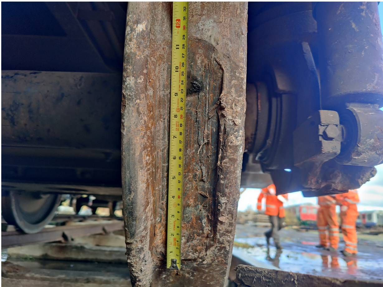
Figure 22: The length of the wheel flats.
