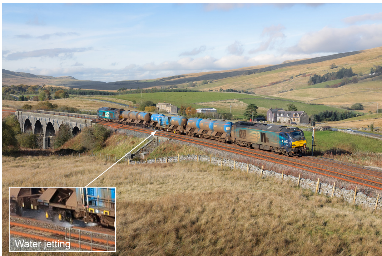
Figure 37: The RHTT on the Settle to Carlisle line on the day before the derailment (courtesy of Aidan Fort).
