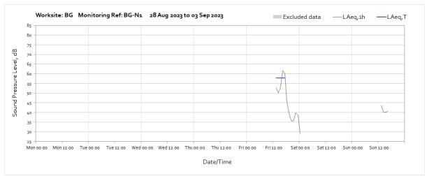
Note: Missing and intermittent data from the beginning of the month until 13:00 on Tuesday 12<sup>th</sup> September is due to power supply problems. A different solar controller Is being obtained.
