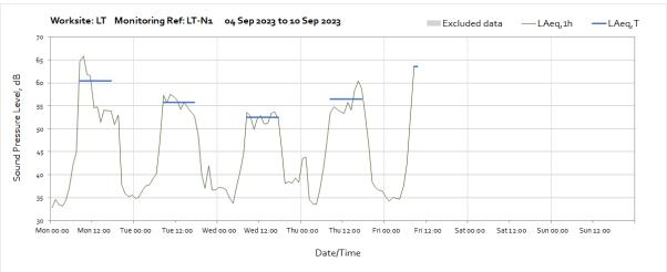
Note: Missing data from 10:00 on Friday 8<sup>th</sup> September onwards was due to problems with the monitor power supply. This problem is being addressed.
