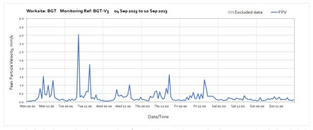
Note: The high vibration levels on Tuesday 5<sup>th</sup> September are due to utility diversion works which included excavating and backfilling within 20m of the monitor.
