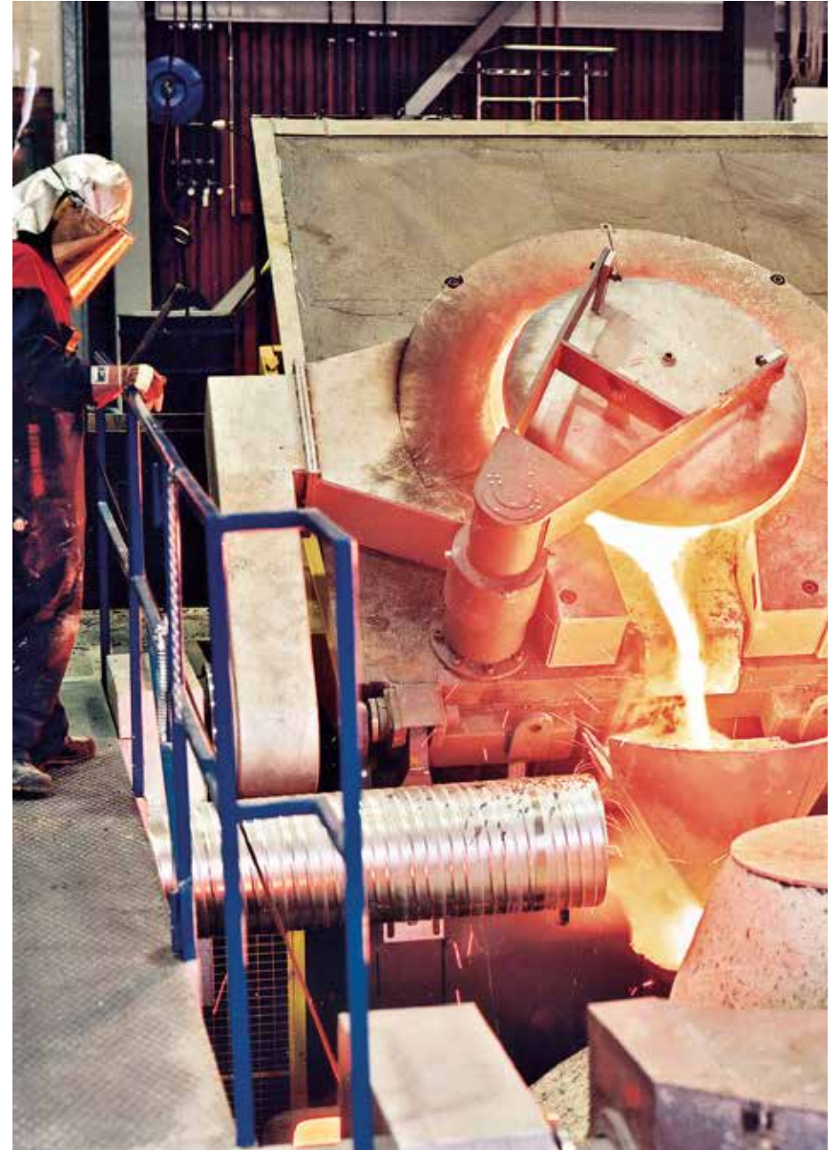
Metallic waste being melted
