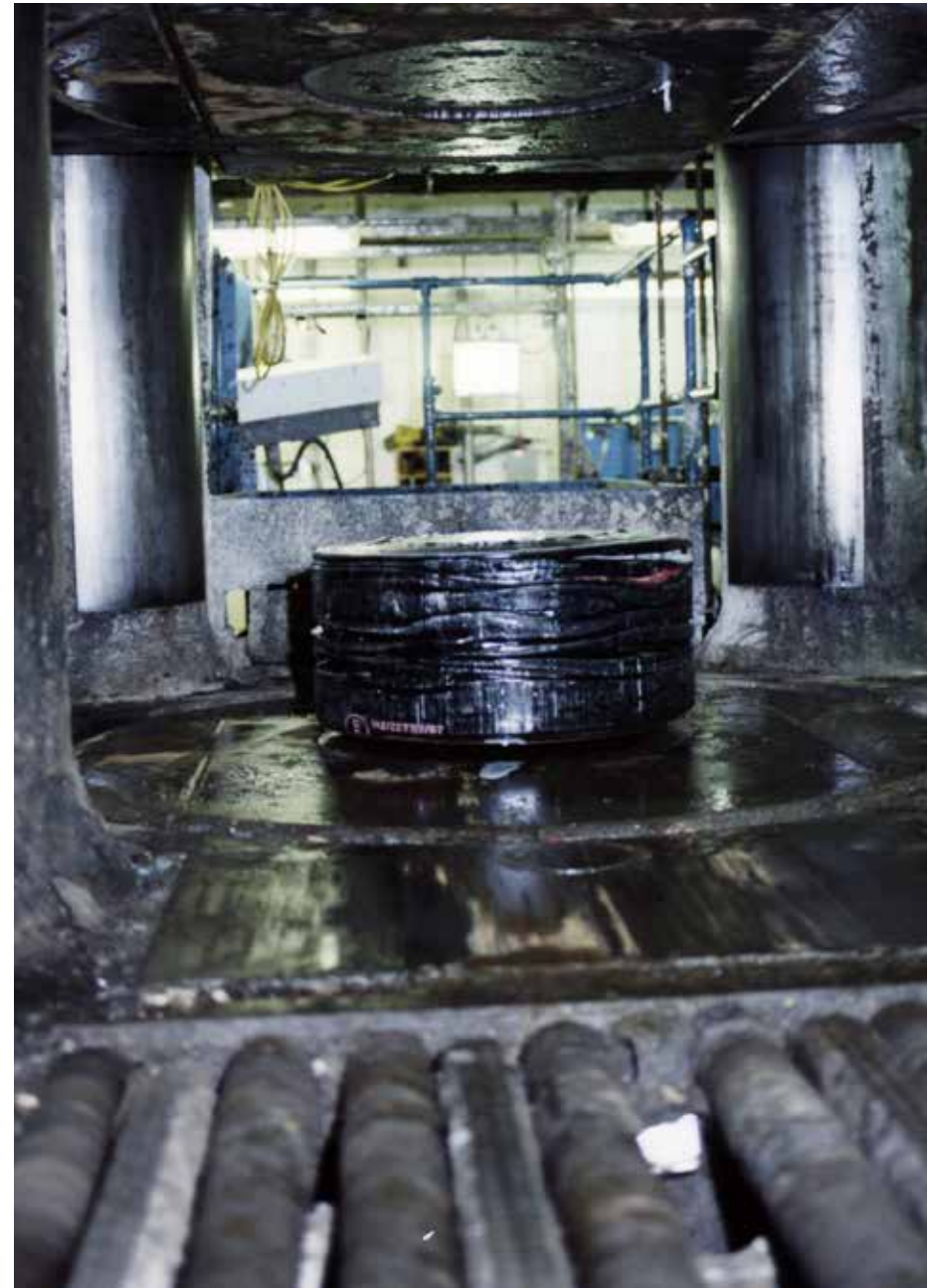
An ILW container being compacted for storage
