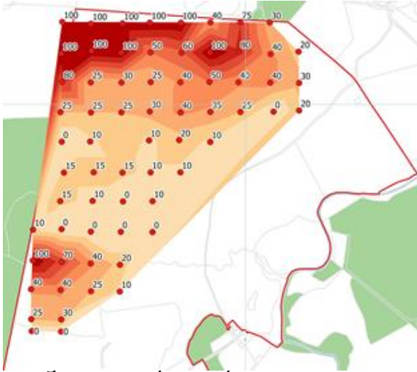
Figure 1 – Example map showing peat resource with peat depth sampling points labelled with corresponding peat depth in cm.
