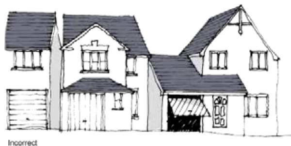
Integral garage doors can be unduly dominant and damage the scale
