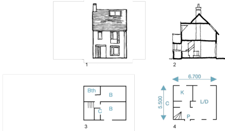
1. Front elevation 2. Section 3. First-floor 4. Ground-floor
