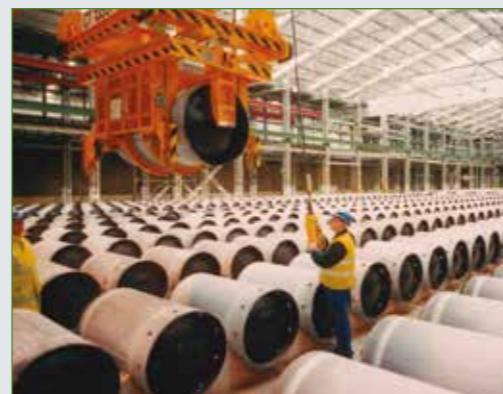
Current uranium storage at Capenhurst
