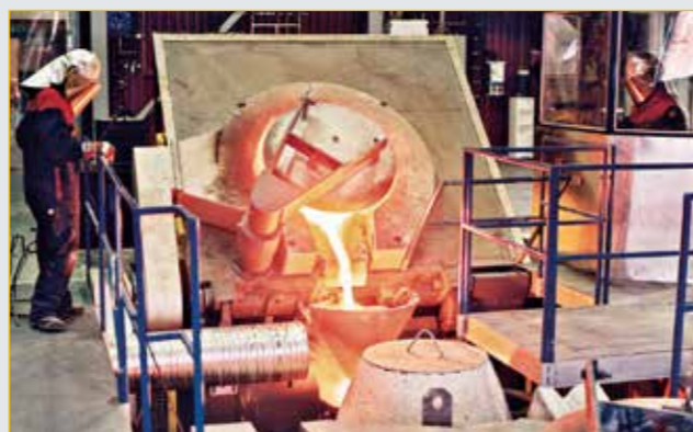
Metal melting - one of the ways of treating LLW
