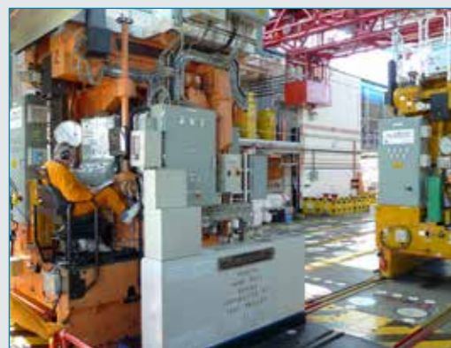
Defueling activity at one of the Magnox stations
