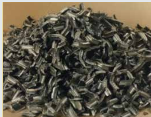
ILW Magnox fuel cladding swarf
