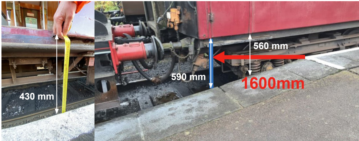
Figure 10: Reconstruction photos showing standard platform stepping height (left) and the increased stepping heights from the train at its stopped position (right).
