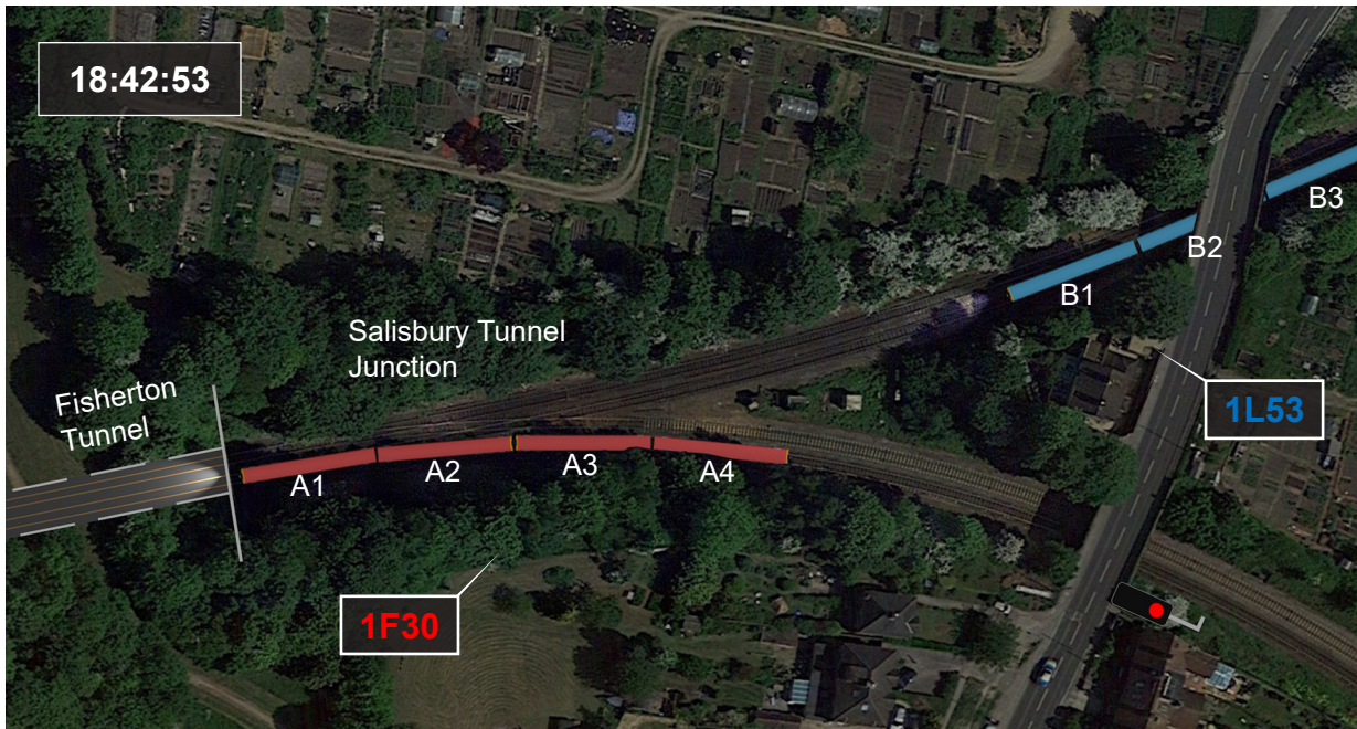
Figure 9. Diagram showing train 1L53 (carriages marked as B1 to B3) and train 1F30 (carriages marked as A1 to A4) immediately before the collision.
