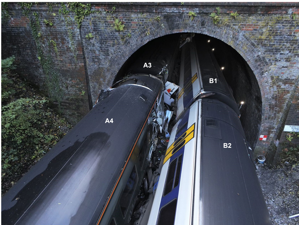
Figure 14: View from London portal of Fisherton Tunnel showing the rear carriages of train 1F30 (A3 and A4) and front carriages of train 1L53 (B1 and B2).
