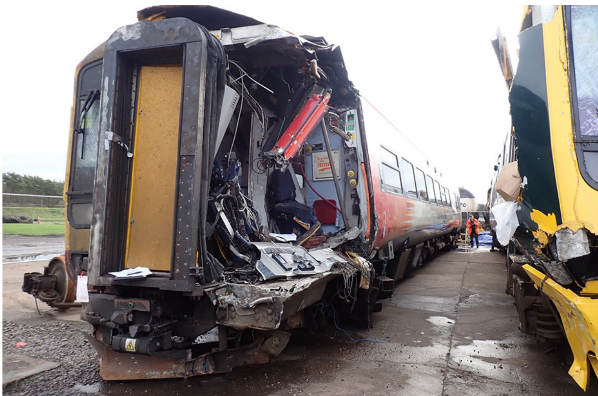
Figure 45: Cab of train 1L53 (additional damage was caused by the fire and rescue service during the extraction of the injured train driver).
