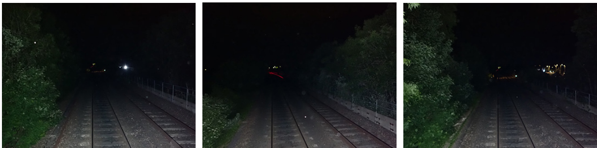
Figure 38: RAIB reconstruction showing the environment on approach to signal SY29: (left) 798 metres from signal SY29; (centre-enhanced) reflection from lighting from signal SY29 at danger on the railhead; and (right) 773 metres from signal SY29 with street lighting and car forecourt lighting visible.
