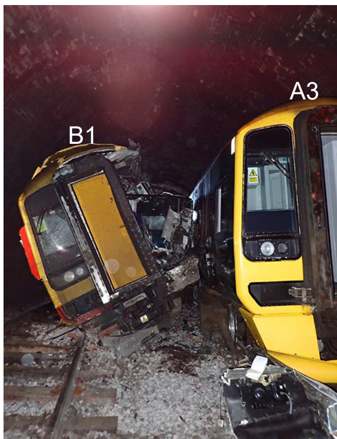
Figure 15: View from within Fisherton Tunnel showing the front cab of train 1L53 (B1) and carriage A3, having separated from carriage A2, of train 1F30. Parts of the driving cab of train 1L53 have been cut away by the emergency services to release the trapped driver.
