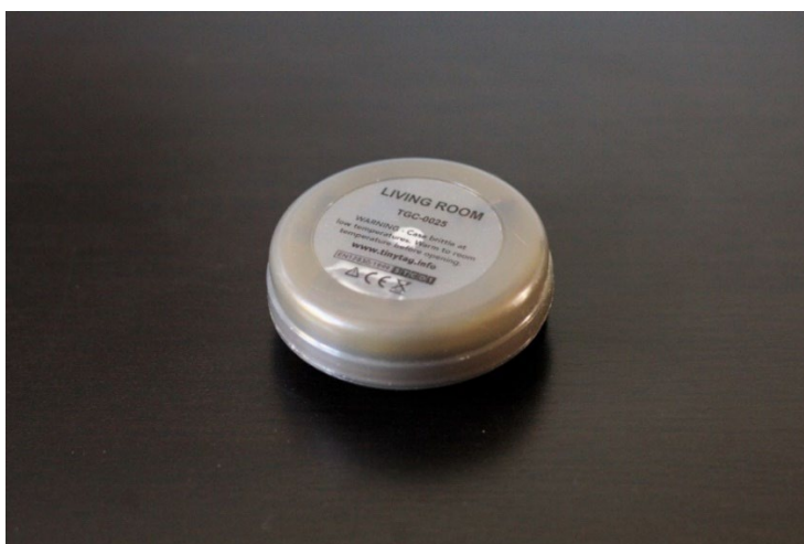
Figure 3.1: Modified Tinytag Transit 2 temperature logger
