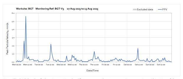
Note: The high levels of vibration on Monday 7<sup>th</sup> August are due to excavation occurring within 20m of the monitor.
