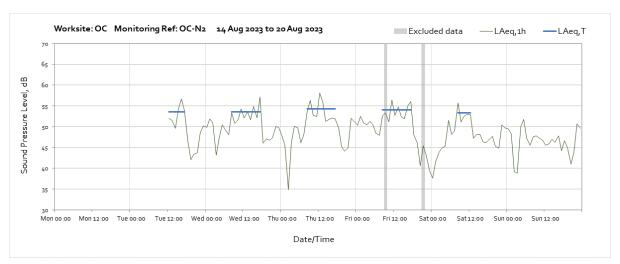
Note: Missing data from 13:00 on Wednesday 9<sup>th</sup> August to 12:00 on Tuesday 15<sup>th</sup> August was due to a damaged cable. The cable has now been replaced.
