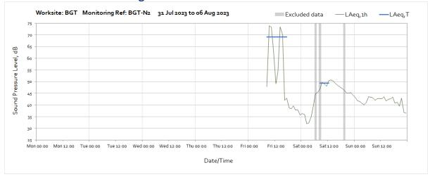
Note: Missing data from the beginning of the month to 09:00 on Friday 4<sup>th</sup> August was due to a power issue arising from difficulty in accessing the monitor. Following de-vegetation work the battery was replaced.
