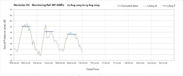
Note: Missing data from 00:00 on Thursday 10<sup>th</sup> August until month end was due to loss of battery power due to a fault with the solar charge controller. A new solar controller is being deployed shortly.
