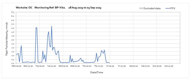
Note: High vibration levels throughout the week were due to embankment works including excavation.
