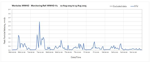
Note: High vibration levels recorded at 11:00 on Tuesday 8<sup>th</sup> August were due to haul road maintenance undertaken close to the monitoring station. The nearest residential receptors are further away and therefore HS2 vibration levels are expected to be lower at the receptors.
