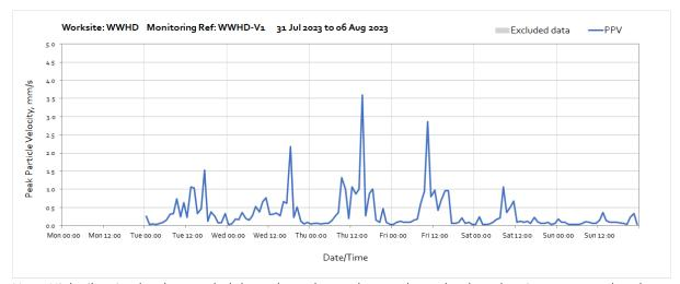
Note: High vibration levels recorded throughout the week were due to haul road maintenance undertaken close to the monitoring station. The nearest residential receptors are further away and therefore HS2 vibration levels are expected to be lower at the receptors.
