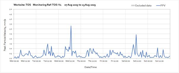
Note: High vibration levels recorded at 13:00 on Wednesday 9<sup>th</sup> August were due to falsework, moving materials, shutters and concrete works undertaken 30m from the monitoring station. The nearest residential receptors are further away and therefore HS2 vibration levels are expected to be lower at the receptors.
